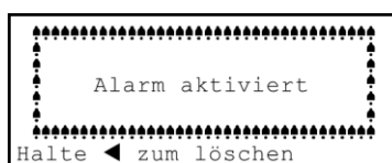
Fig. 85 The LCD display as an alarm is raised from the Hub
